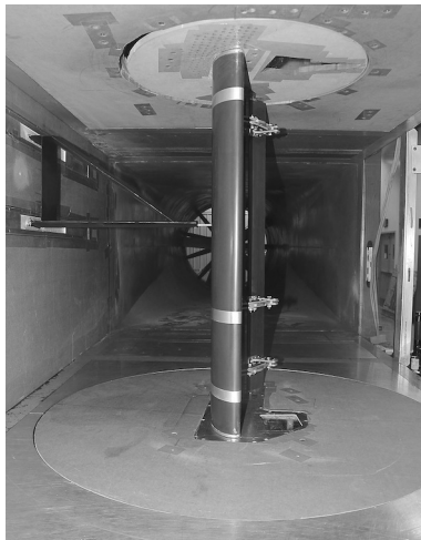
Figure 6. Experimental setup of sidewall-mounted traverse with three-element airfoil model installed.
