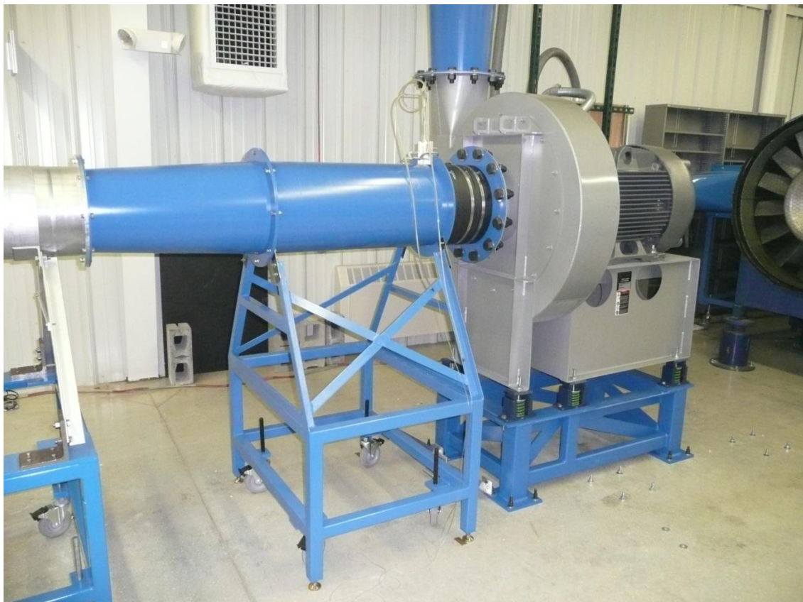
Fig. 2.5 Centrifugal blower with ducting and support frames.
