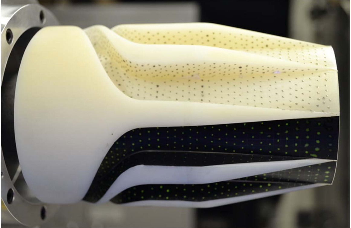
Fig. 2.28. Vaned model prepared for both fluorescent and lampblack based surface oil flow visualization.
