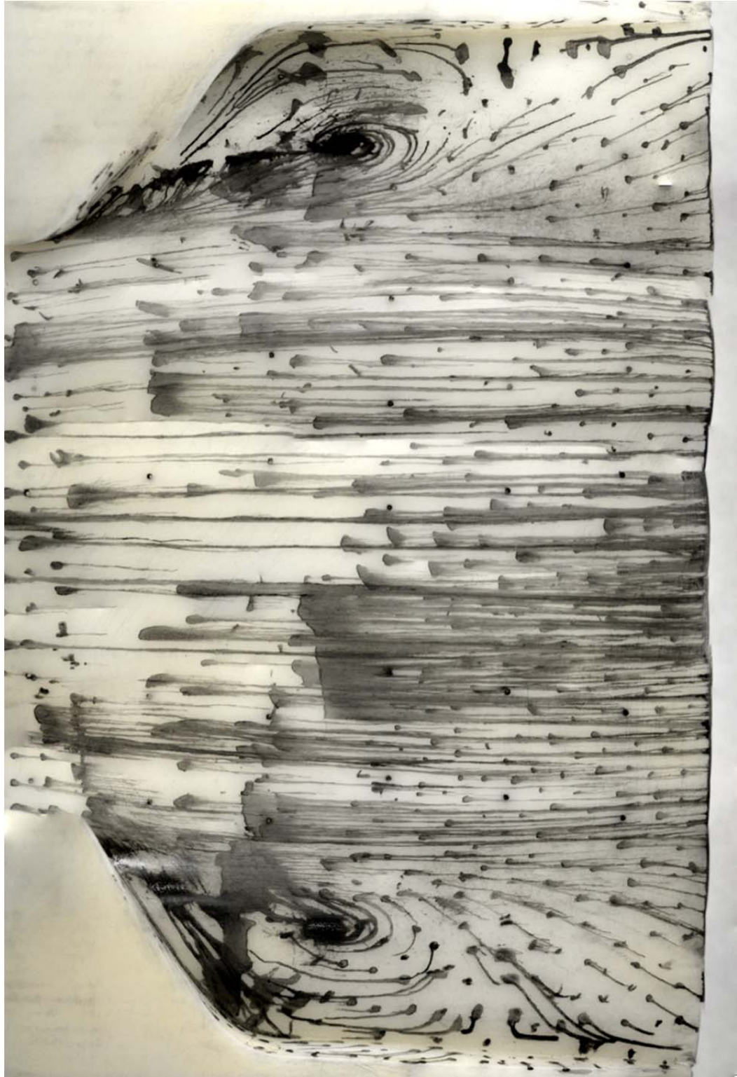
Fig. 3.43. Clean model lampblack surface oil flow visualization at M_{tunnel} = 0.704 . Model surface is unwrapped, showing clear model symmetry.
