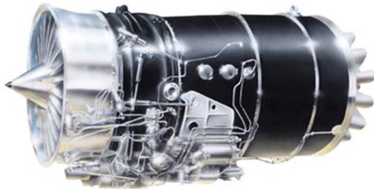
Fig. 1.6. The Rolls Royce Tay turbofan. Courtesy of RR.
