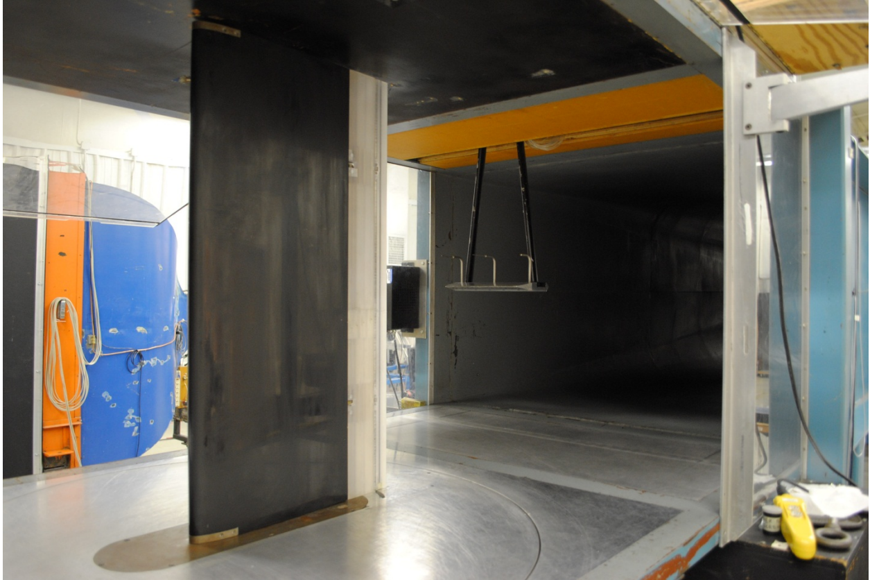
Fig. 2.9 Wake rake and NACA 3415 model installed in test section.
