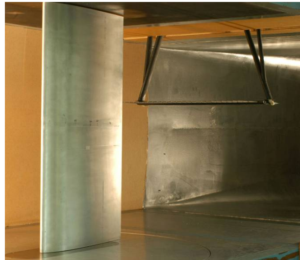
Fig. 2 Photograph of subscale NACA 23012 airfoil model installed in Illinois wind-tunnel test section.
