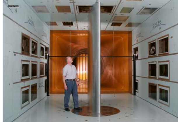
Fig. 1 Photograph of full-scale NACA 23012 airfoil model installed in ONERA F1 wind-tunnel test section.
