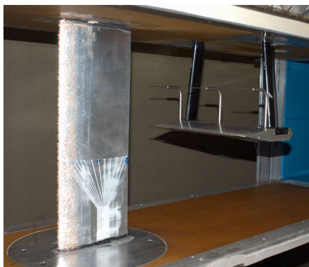
Fig. 4 Wake rake installed behind 50% blade section airfoil model with ice simulation of Run 19A installed on leading edge.
