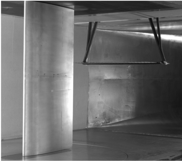
Fig. 1 Traversable wake rake installed behind the NACA 23012 airfoil model.
