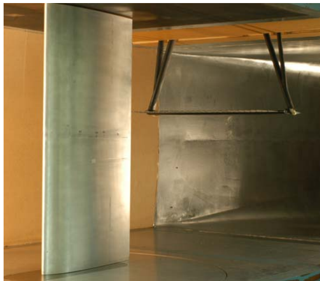
Fig. 1 Wake rake installed behind NACA 23012 airfoil model.
