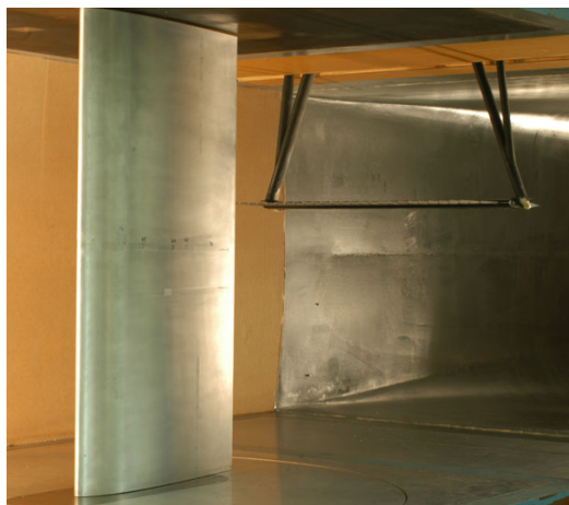
Fig. 1 Traversable wake rake installed behind NACA 23012 model.
