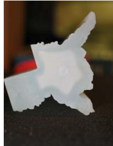
Fig. 2. Cross-section of an alternate leading edge. Picture is showing one end of the simulated ice accretion, corresponding to IRT run 58.
