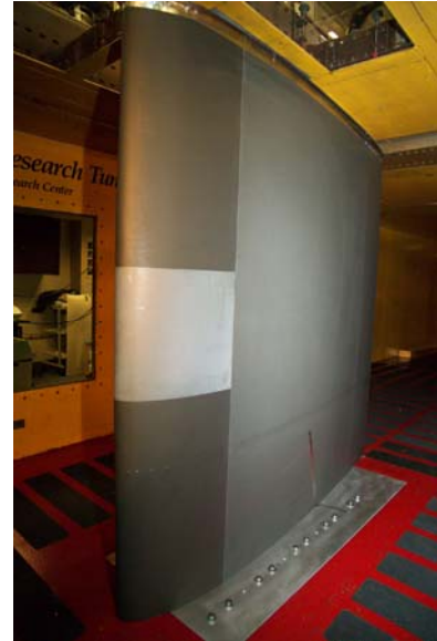
Fig. 16 Full-scale NACA 23012 ice accretion model installation in NASA IRT.
