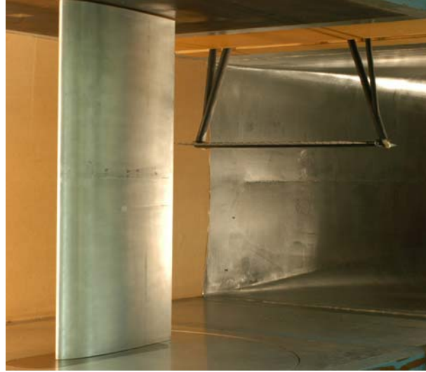
Fig. 8 Subscale NACA 23012 aerodynamic model installation in University of Illinois wind tunnel.
