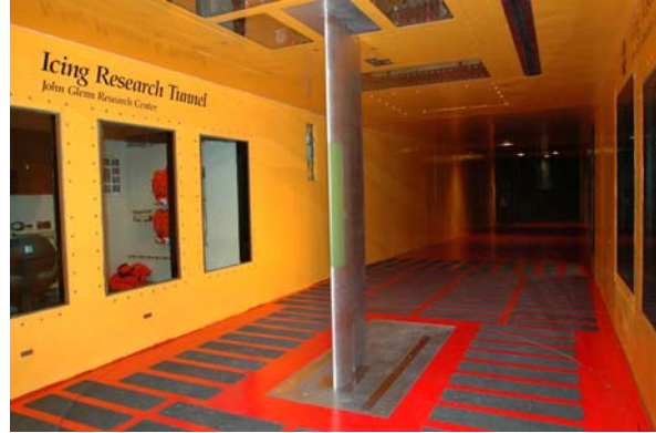
Fig. 2 Subscale NACA 23012 ice accretion model installation in NASA IRT.
