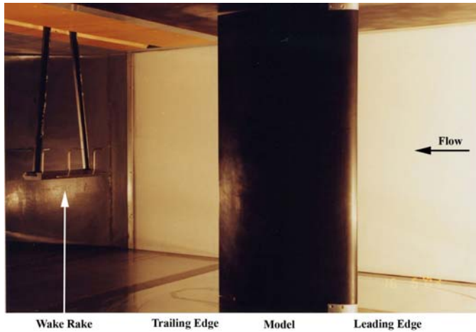
Fig. 1 Experimental setup in the UIUC 3' x 4' wind tunnel.
