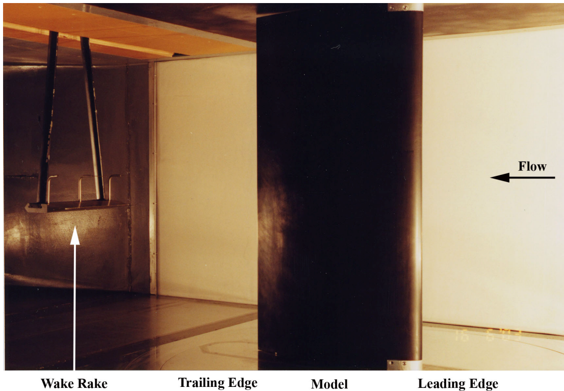
Figure 13. Experimental set-up for aerodynamic testing.
